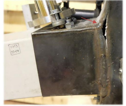
Figure 12: FM3 steel cuff failure.
